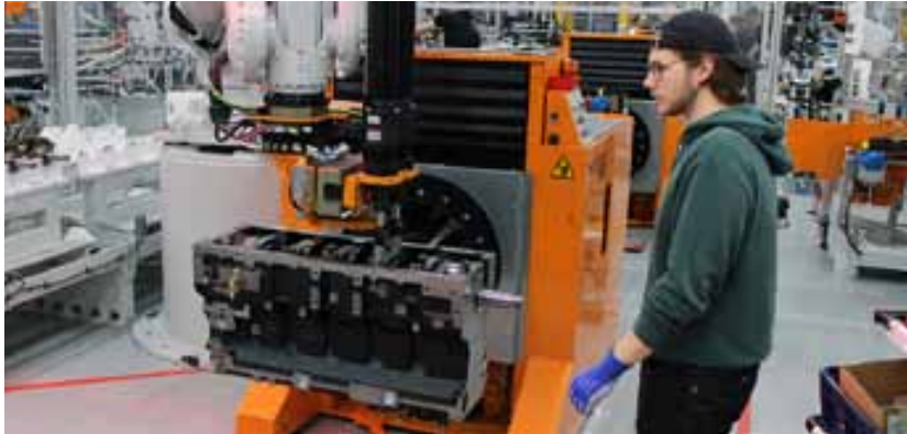
Mechanic Julius Salmela installs a crankshaft with the help of an industrial robot.
