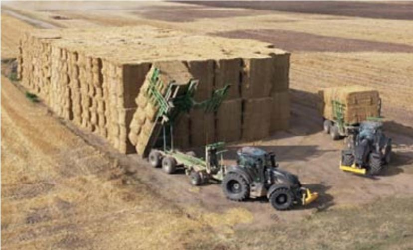
Valtra T234 Direct tractors were ideal for operating the Heath bale chasers. Cambridgeshire-based AgriBale operated a fleet of 17 Valtra T4-series tractors last harvest – baling and transporting 60,000t of straw.
