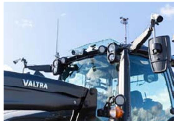
Cameras mounted on the outside show the operator what is happening around the tractor.
