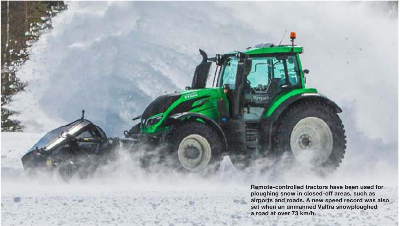
Remote-controlled tractors have been used for ploughing snow in closed-off areas, such as airports and roads. A new speed record was also set when an unmanned Valtra snowploughed a road at over 73 km/h.
