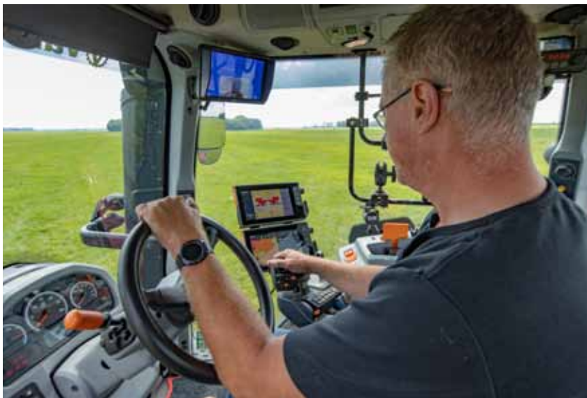
With two small SmartTouch screens, the view to the outside remains optimal. All the data and settings of the tractor and implement are within reach. The screen at the top is from a monitoring camera.
