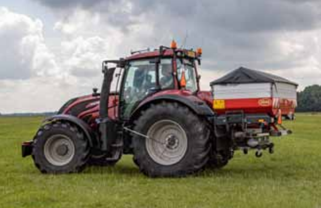
The Valtra T174 Direct from Thijssen has Michelin XeoBib tyres with tyre pressure control for minimum ground pressure.
