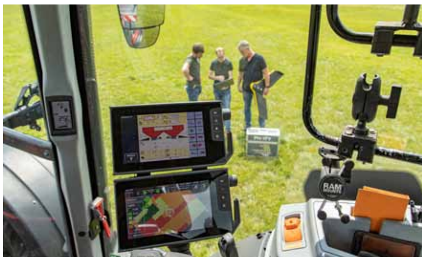
Height maps and scans of crop growth are used to create fertilising plans. The lower part of this section in blue has experienced flooding, which means that crop growth there is lagging behind (yellow-red areas on the NDVI map). Agronomically, a higher fertiliser dose in the better places marked in green provides the highest return.
