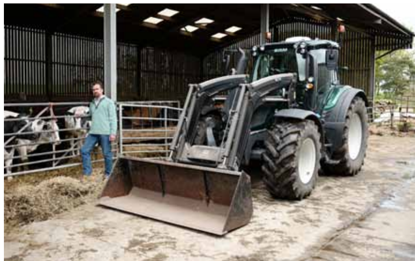
The Valtra N174 Versu is equipped with a front loader, mainly for loading bale trailers in the field.
