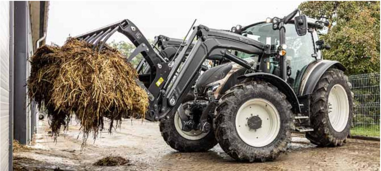
The G Series weighs 5140 kg. The light weight, compact size and agile performances makes it ideal for farm tasks. The maximum total weight is 9500 kg.
