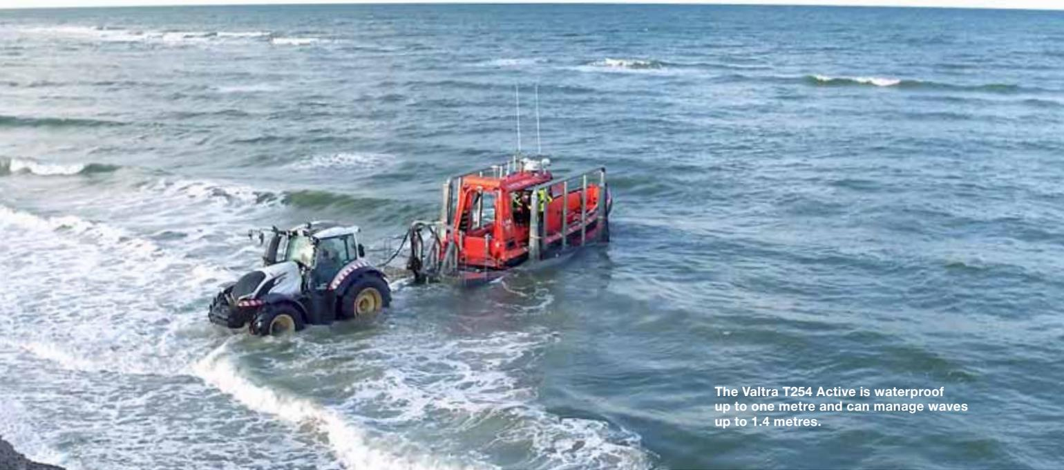
The Valtra T254 Active is waterproof up to one metre and can manage waves up to 1.4 metres.
