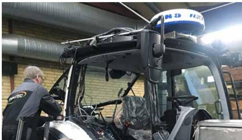
The Valtra N154 is a multipurpose machine that can be fitted with a wide range of tools, including a maritime radar, an infrared heatseeking camera and a search spotlight.
