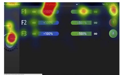
The eye movements of testers were tracked while using SmartTouch using special cameras, allowing developers to see whether users found the functions they were looking for and understood the icons.
