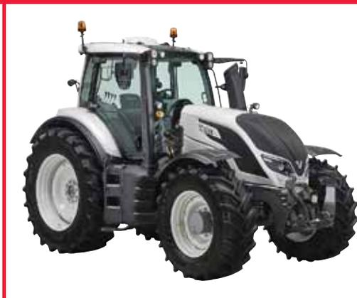
The new T and N Series models can be identified by their narrower exhaust pipes, which allow better visibility from the cab.
