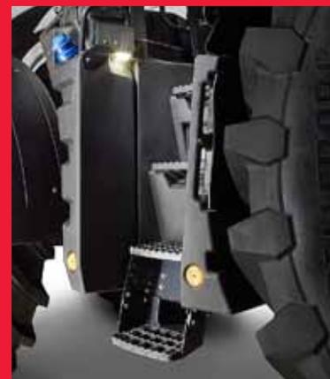
On the right: Access to the cab of S Series models has been made easier, and there is more space inside the cab for small items.
