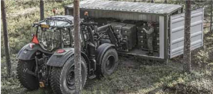
Supplies are delivered to Finnish troops in the field in containers transported by Valtra tractors. The same tractors can also be used to maintain roads, plough snow and load or unload supplies, as well as for preparing fortifications.
