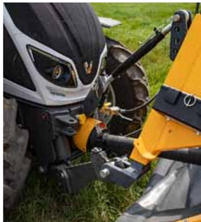
The new A Series can be fitted with a front linkage or front PTO at the Unlimited Studio.
