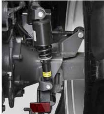
The mechanical cab suspension is adjustable and uses double Panhard rods to stabilise the cab.
