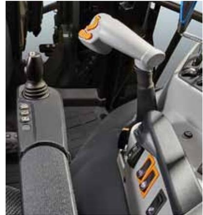
The transmission is easy to use thanks to the ergonomic lever and rocker switches.
