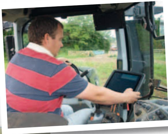
The Auto-Guide controls are conveniently located and easily set. David has also installed a TV monitor that is used in conjunction with a remote camera at the rear of balers or planters to check operations. The cab is also fitted with a hands-free mobile phone and a CB radio to keep him in contact with home and colleagues.
