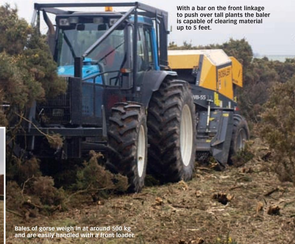
With a bar on the front linkage to push over tall plants the baler is capable of clearing material up to 5 feet.
