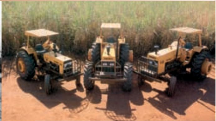
▲ Valmet do Brasil's "Alcool" series featured three models: the four-cylinder Valmet 88 and the six-cylinder Valmet 118 and 118-4.
