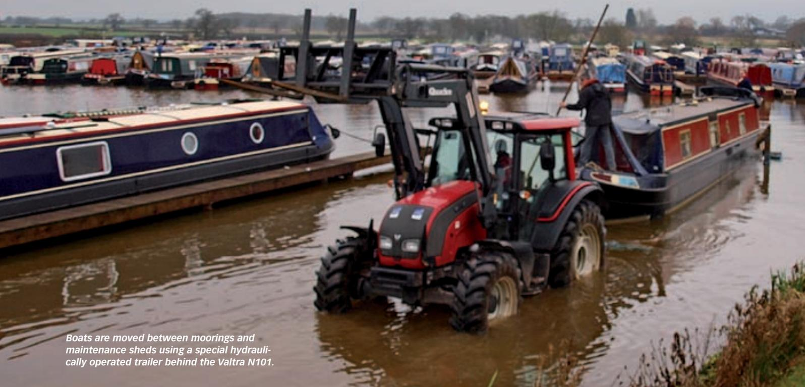
*Boats are moved between moorings and maintenance sheds using a special hydraulically operated trailer behind the Valtra N101.*
