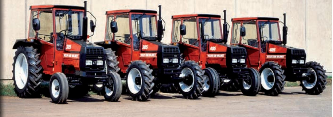
*The Volvo BM Valmet 305-4/405-4 was an excellent general-use tractor. Depending on the tyre specifications, the tractor weighed 3,200-3,300 kilos. The transmission featured 8+4R fully synchronised gears, and a creeper gear was also available, making for 12+8R gears.*
