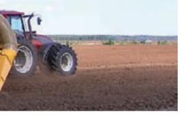
Cutter peat accounts for the majority of production. The top layer of peat, around one inch in thickness, is first turned over and dried using a cutter and turner. After this the dry peat is loaded onto a peat trailer by suction or mechanically.
