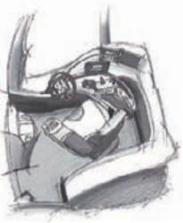
Valtra has a long tradition of developing user friendly, ergonomic and comfortable tractors. The safety cab, synchronised transmission, gear levers on the right, hydrostatic steering, handbrake integrated with the shuttle and many other features that one takes for granted today were introduced to the tractor world by Valtra and its predecessors Valmet and Volvo BM. Valtra Design Manager Kimmon Wihinen is doing his part to ensure that this heritage is continued in Valtra's future tractor models.
