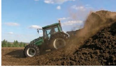
Tractors also have to versatile and agile for working on peat bogs. Here a Valtra N tractor is stacking peat for storage. This model offers excellent ground clearance, good protection and filtering, and the benefits of the TwinTrac reverse-drive system.
