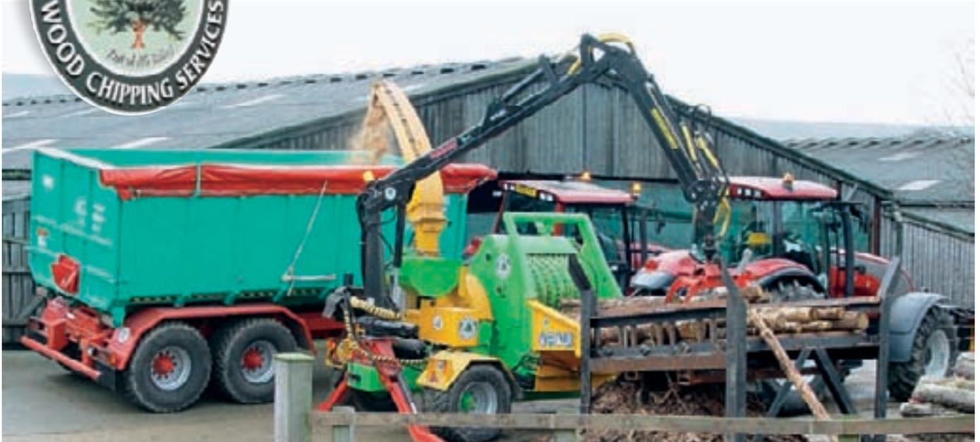
*For maximum output Denton Park Estate uses a telehandler to load a table with rollers, ensuring the chipper has a constant supply of timber for maximum output – cut chips can be loaded into trailers or blown into store.*
