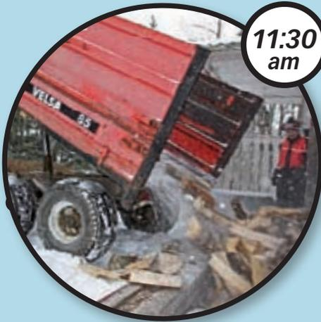
Around ten loosely stacked cubic metres of logs have been loaded in the trailer and are then emptied through a hatch into the cellar of the house. The wood is used to heat the house, water, oven and sauna. The large cellar can store up to 20 cubic metres of wood alongside the stove and a 2,000-litre boiler.
