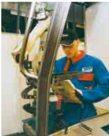
Robot welder Arto Niemelä checks that the co-ordinates of the welding robot have not changed during the holidays.
