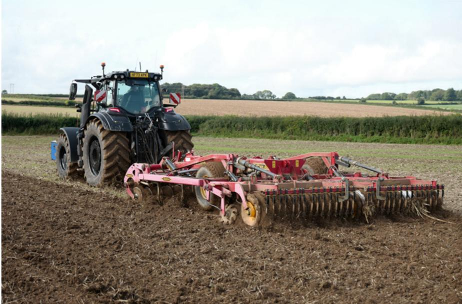
Andy says that the CVT transmission allows him to make the most of the power available and main-tain optimum work rates in variable conditions.
