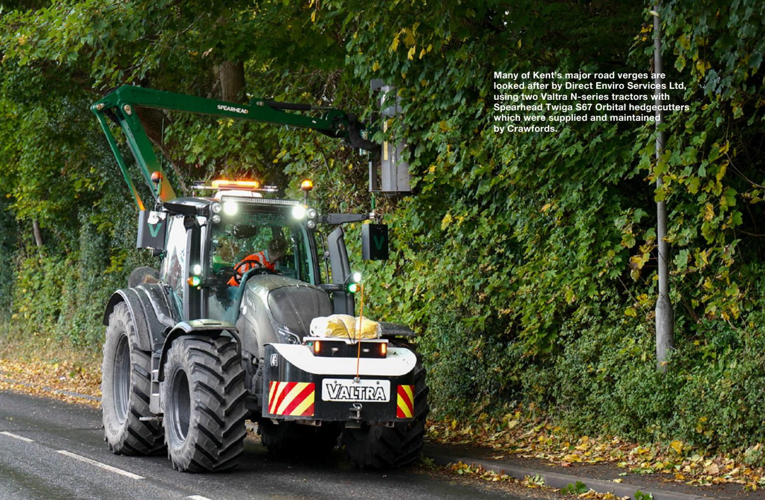
Many of Kent's major road verges are looked after by Direct Enviro Services Ltd, using two Valtra N-series tractors with Spearhead Twiga S67 Orbital hedgecutters which were supplied and maintained by Crawfords.
