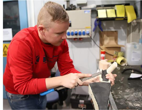
Industrial Designer Henri Hokkanen works on a plastic model of an armrest. A lot of plastic, wood and 3D-printed components are used in the design studio to make full-size mock-up models of future tractors and cabs.
