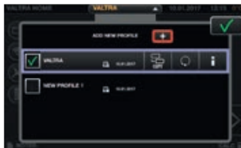
Profiles for operators and implements which can be easily changed from any screen menu. All the setting changes will be saved in the selected profile.
