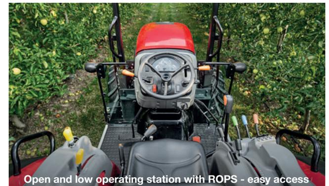
Open and low operating station with ROPS - easy access
